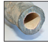
*Yog ibyam kob lub npe hu Phosphate txuag tiv thaiv raj dej sab hauv kom tsis txhob ntawm muaj kauv xeb.
